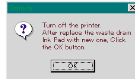
Figure 5-41. Replace the Waste drain in pad & Set the market setting
