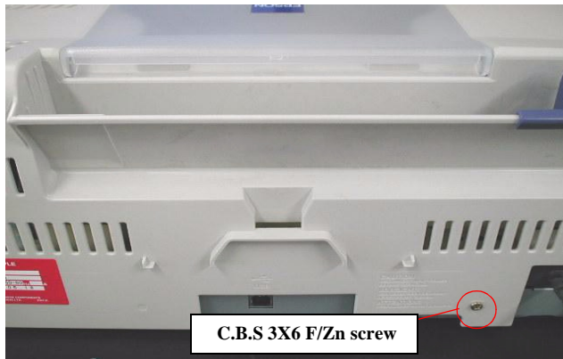
Figure 4-3. Removing 1screw for Housing
