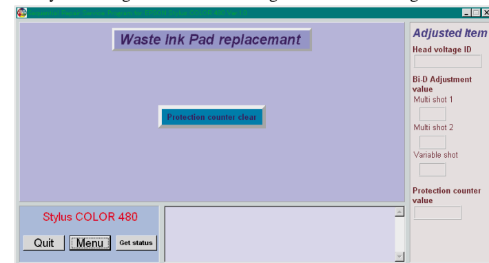
Figure 5-49. Waste drain ink pad replacement
